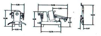
NASCOMATIC 2001-6 AUTOMATIC SCREWFEEDING SYSTEM FOR SMALL SCREWS #0 - #4
